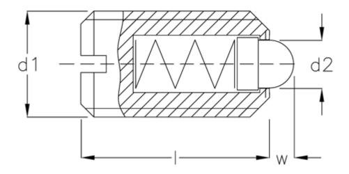
$\begin{array}{ll} d1 & = M8 \\ d2 & = 3.8 \\ Length I & = 16 \\ Spring pressure N bottom = 59.0 \\ Spring pressure N top & = 23.0 \\ W & = 2.0 \end{array}$
